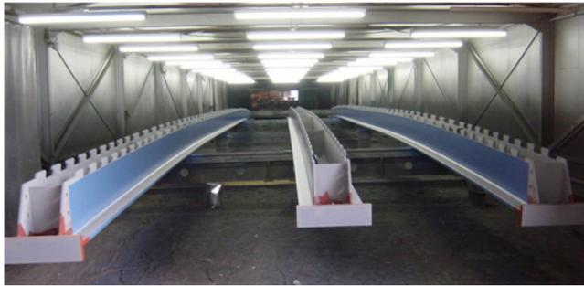
Fig. 4 – Rolled girders after cutting and coating in the shop
