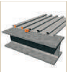
Placing of filler plugs
