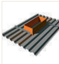
Box-out using steel formwork
