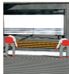
Laying of the floor decks
