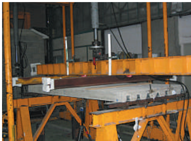
Composite slab tests Composite stage
