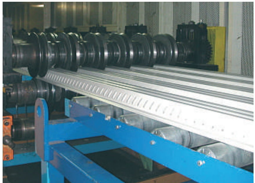
Fabrication of a composite floor deck
