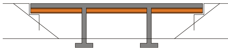
Figure 1-10: Multi span semi-integral abutment bridge
