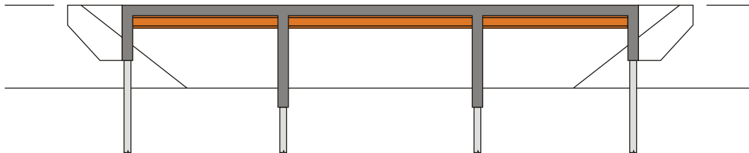
Figure 1-9: Multi span integral abutment bridge
