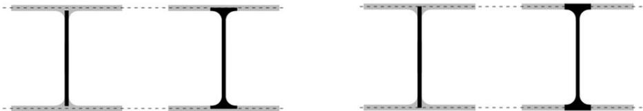
Figure 5.2 Definition of web and strong axis shear area in rolled I-shaped sections, from left to right:  $A_w$  EN 1993-1-1,  $A_v$  EN 1993-1-1,  $A_v$  DIN 18800,  $A_v$  NEN 6770
