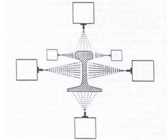
Figure 18 – Spray configuration in rail cooling system
