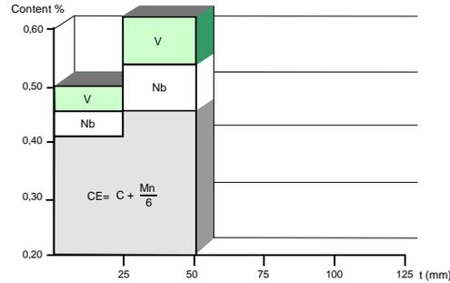
Figure 5 – Steel alloying contents for S460, controlled rolling
