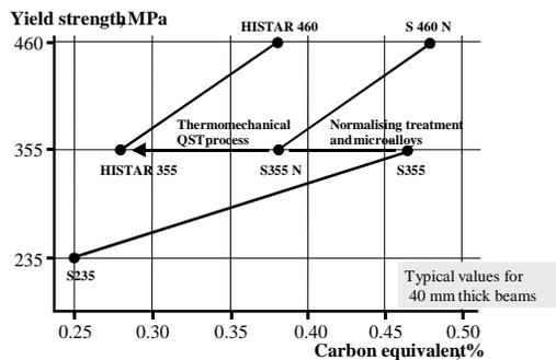
Figure 11 – Evolution of the yield strength in function of CE
