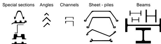
Figure 1 – Hot rolled sections
