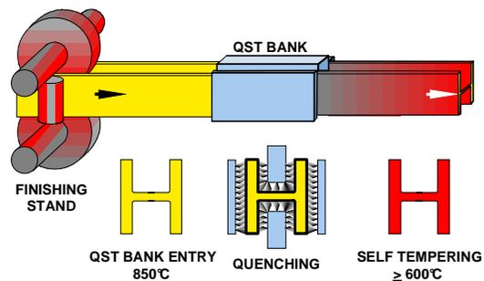
Figure 6 – QST process applied on beams in the rolling heat
