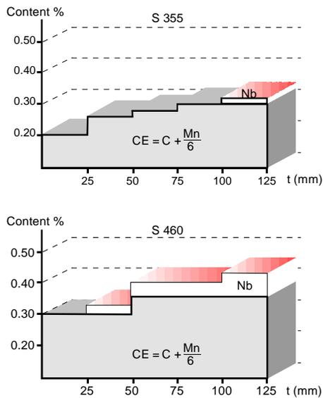
Figure 10 - Steel alloying concept for the production of QST structural shapes
