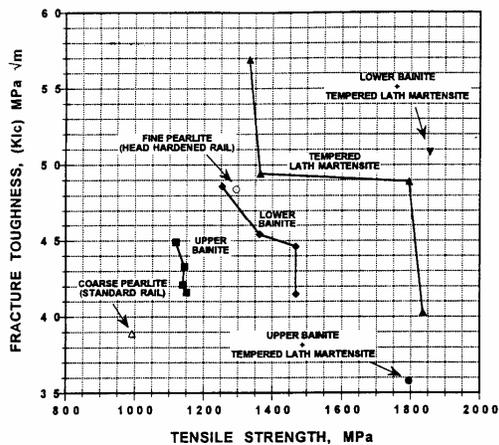
Figure 21 – Fracture toughness/tensile strength plot of rails
